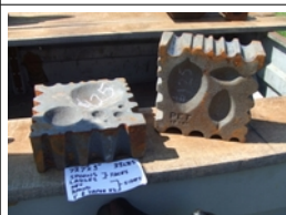
Swedge Block 7"x7"x3" on faces - spoons and ladles and on sides - hex, round, V & Taper round cost $125.00
